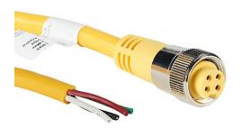
ZIPport connection cable, 7/8in - 16 UN2 thread nut 4-pin female axial to pigtail with North American color code, PVC outer jacket, yellow, nickel-plated brass connector, 6.5ft/2m cable length, IP67.
