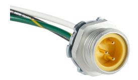
ZIPport bulkhead connector, 7/8in 3-pin male to pigtail, 16 AWG, 0.9ft/0.3m cable length, ether-based polyurethane conductor insulation material, IP67.
