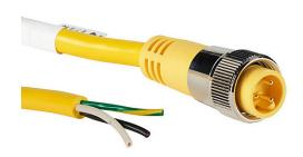
ZIPport connection cable, 7/8in - 16 UN2 thread nut 3-pin male axial to pigtail with North American color code, PVC outer jacket, yellow, nickel-plated brass connector, 19.6ft/6m cable length, IP67.
