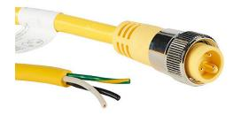
ZIPport connection cable, 7/8in - 16 UN2 thread nut 3-pin male axial to pigtail with North American color code, PVC outer jacket, yellow, nickel-plated brass connector, 13.1ft/4m cable length, IP67.
