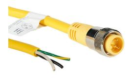
ZIPport connection cable, 7/8in - 16 UN2 thread nut 3-pin male axial to pigtail with North American color code, PVC outer jacket, yellow, nickel-plated brass connector, 6.5ft/2m cable length, IP67.
