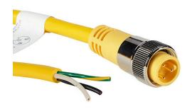
ZIPport connection cable, 7/8in - 16 UN2 thread nut 3-pin male axial to pigtail with North American color code, PVC outer jacket, yellow, nickel-plated brass connector, 32.8ft/10m cable length, IP67.
