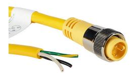
ZIPport connection cable, 7/8in - 16 UN2 thread nut 3-pin male axial to pigtail with North American color code, PVC outer jacket, yellow, nickel-plated brass connector, 32.8ft/10m cable length, IP67.
