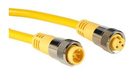
ZIPport connection cable, 7/8in - 16 UN2 thread nut 3-pin male axial to 7/8in - 16 UN2 thread nut 3-pin female axial, PVC outer jacket, yellow, nickel-plated brass connector, 19.6ft/6m cable length, IP67.
