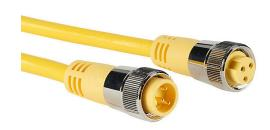
ZIPport connection cable, 7/8in - 16 UN2 thread nut 3-pin male axial to 7/8in - 16 UN2 thread nut 3-pin female axial, PVC outer jacket, yellow, nickel-plated brass connector, 13.1ft/4m cable length, IP67.
