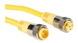
ZIPport connection cable, 7/8in - 16 UN2 thread nut 3-pin male axial to 7/8in - 16 UN2 thread nut 3-pin female axial, PVC outer jacket, yellow, nickel-plated brass connector, 6.5ft/2m cable length, IP67.
