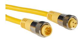
ZIPport connection cable, 7/8in - 16 UN2 thread nut 3-pin male axial to 7/8in - 16 UN2 thread nut 3-pin female axial, PVC outer jacket, yellow, nickel-plated brass connector, 32.8ft/10m cable length, IP67.
