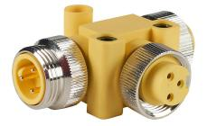
ZIPport T-coupler, (2) 3-pole female 7/8in - 16 UN2 nuts to 3-pole male 7/8in - 16 UN2 barrel, parallel distribution.
