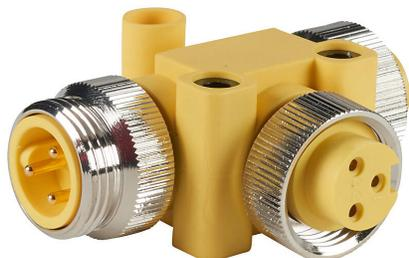
ZIPport T-coupler, (2) 3-pole female 7/8in - 16 UN2 nuts to 3-pole male 7/8in - 16 UN2 barrel, parallel distribution.
