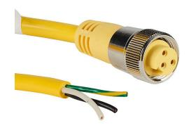
ZIPport connection cable, 7/8in - 16 UN2 thread nut 3-pin female axial to pigtail with North American color code, PVC outer jacket, yellow, nickel-plated brass connector, 13.1ft/4m cable length, IP67.
