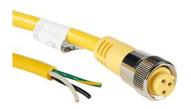
ZIPport connection cable, 7/8in - 16 UN2 thread nut 3-pin female axial to pigtail with North American color code, PVC outer jacket, yellow, nickel-plated brass connector, 6.5ft/2m cable length, IP67.
