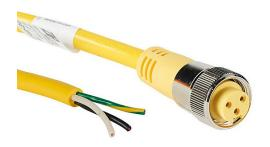
ZIPport connection cable, 7/8in - 16 UN2 thread nut 3-pin female axial to pigtail with North American color code, PVC outer jacket, yellow, nickel-plated brass connector, 32.8ft/10m cable length, IP67.
