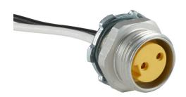
ZIPport bulkhead connector, 7/8in 2-pin female to pigtail, 16 AWG, 0.9ft/0.3m cable length, ether-based polyurethane conductor insulation material, IP67.
