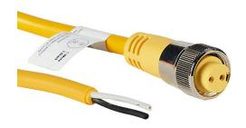
ZIPport connection cable, 7/8in - 16 UN2 thread nut 2-pin female axial to pigtail with North American color code, PVC outer jacket, yellow, nickel-plated brass connector, 19.6ft/6m cable length, IP67.
