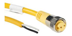
ZIPport connection cable, 7/8in - 16 UN2 thread nut 2-pin female axial to pigtail with North American color code, PVC outer jacket, yellow, nickel-plated brass connector, 13.1ft/4m cable length, IP67.
