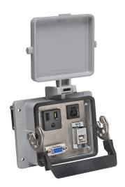
ZIPport panel interface connector, single 120 VAC outlet, (1) 9-pin D-sub connector with female exterior/male interior, (1) USB B port with female exterior/USB A female interior, 3A circuit breaker.
