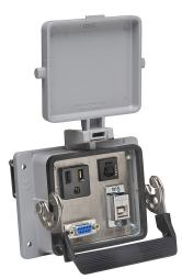
ZIPport panel interface connector, single 120 VAC outlet, (1) 9-pin D-sub connector with female exterior/male interior, (1) USB B port with female exterior/USB A female interior, 3A circuit breaker.
