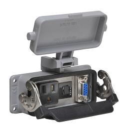
ZIPport panel interface connector, single 120 VAC outlet, (1) 9-pin D-sub connector with female exterior/male interior, 3A circuit breaker.
