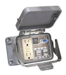
ZIPport panel interface connector, GFCI duplex 120 VAC outlet, (1) 9-pin D-sub connector with female exterior/male interior, (1) USB B port with female exterior/USB A female interior, (1) USB A port with female exterior/USB B female interior.
