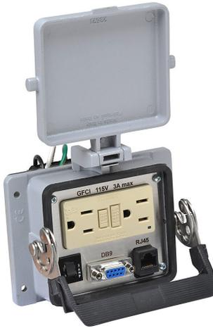
ZIPport panel interface connector, GFCI duplex 120 VAC outlet, (1) 9-pin D-sub connector with female exterior/male interior, (1) RJ45 Ethernet port with female exterior/female interior, 3A circuit breaker.
