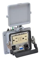
ZIPport panel interface connector, GFCI duplex 120 VAC outlet, (1) 9-pin D-sub connector with female exterior/male interior, (1) RJ45 Ethernet port with female exterior/female interior, 3A circuit breaker.
