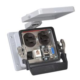
ZIPport panel interface connector, duplex 120 VAC outlet, (1) 9-pin D-sub connector with female exterior/male interior, (1) RJ12 6-pin port with female exterior/RJ12 6-pin female interior, (1) USB A port with female exterior/USB A female interior.
