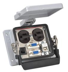
ZIPport panel interface connector, duplex 120 VAC outlet, (2) 9-pin D-sub connectors with female exterior/male interior, (1) USB B port with female exterior/USB A female interior, 3A circuit breaker.
