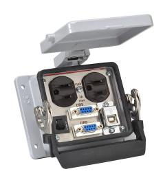
ZIPport panel interface connector, duplex 120 VAC outlet, (2) 9-pin D-sub connectors with female exterior/male interior, (1) USB B port with female exterior/USB A female interior, 3A circuit breaker.
