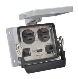
ZIPport panel interface connector, duplex 120 VAC outlet, (1) 9-pin D-sub connector with female exterior/Data Highway 3-pin terminal block interior, (1) RJ45 Ethernet port with female exterior/female interior, 3A circuit breaker.
