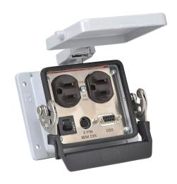
ZIPport panel interface connector, duplex 120 VAC outlet, (1) 9-pin D-sub connector with female exterior/Data Highway 3-pin terminal block interior, (1) 8-pin mini-DIN female exterior/Data Highway 3-pin terminal block interior, 3A circuit breaker.
