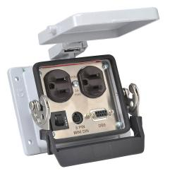
ZIPport panel interface connector, duplex 120 VAC outlet, (1) 9-pin D-sub connector with female exterior/Data Highway 3-pin terminal block interior, (1) 8-pin mini-DIN female exterior/Data Highway 3-pin terminal block interior, 3A circuit breaker.
