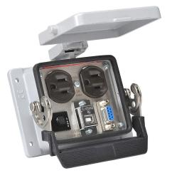
ZIPport panel interface connector, duplex 120 VAC outlet, (1) 9-pin D-sub connector with female exterior/male interior, (1) USB B port with female exterior/USB A female interior, 3A circuit breaker.
