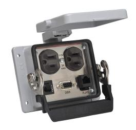
ZIPport panel interface connector, duplex 120 VAC outlet, (1) 9-pin D-sub connector with female exterior/9-position screw terminal block interior, (1) RJ45 Ethernet port with female exterior/female interior, 3A circuit breaker.
