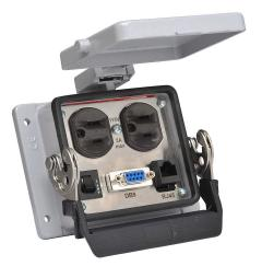
ZIPport panel interface connector, duplex 120 VAC outlet, (1) 9-pin D-sub connector with female exterior/male interior, (1) RJ45 Ethernet port with female exterior/female interior, 3A circuit breaker.
