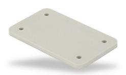
ZIPport bulkhead cutout blank cover plate, thermoplastic, RAL 7044 gray. For use with ZIPport size 6B bulkhead cutouts. Gasket included.
