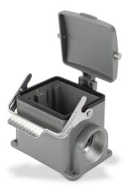
ZIPport surface mount housing, single lever, standard, connector housing size 32B, (2) Pg 36 threaded holes, heavy-duty die cast aluminum. For use with ZIPport size 32B 2-peg connector housings.
