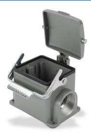
ZIPport surface mount housing, single lever, standard, connector housing size 32B, (2) Pg 36 threaded holes, heavy-duty die cast aluminum. For use with ZIPport size 32B 2-peg connector housings.
