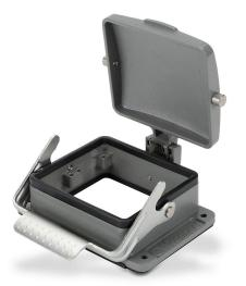
ZIPport bulkhead housing, single lever, automatic closing, connector housing size 32B, heavy-duty die cast aluminum. For use with ZIPport size 32B 2-peg connector housings.
