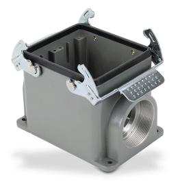
ZIPport surface mount housing, double lever, connector housing size 32B, (2) Pg 36 threaded holes, heavy-duty die cast aluminum. For use with ZIPport size 32B 4-peg connector housings.
