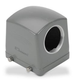
ZIPport hood housing, 4-peg, side entry, connector housing size 32B, (1) Pg 36 threaded hole, heavy-duty die cast aluminum. For use with ZIPport size 32B double lever connector housings.
