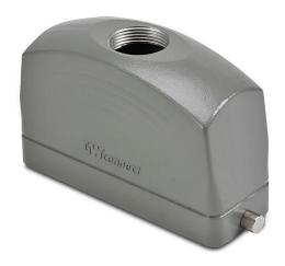
ZIPport hood housing, 2-peg, top entry, connector housing size 24B, (1) Pg 21 threaded hole, high construction, heavy-duty die cast aluminum. For use with ZIPport size 24B single lever connector housings.
