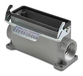
ZIPport surface mount housing, single lever, connector housing size 24B, (2) Pg 29 threaded holes, high construction, heavy-duty die cast aluminum. For use with ZIPport size 24B 2-peg connector housings.
