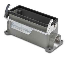
ZIPport surface mount housing, single lever, connector housing size 24B, (2) Pg 21 threaded holes, heavy-duty die cast aluminum. For use with ZIPport size 24B 2-peg connector housings.
