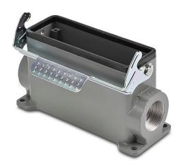
ZIPport surface mount housing, single lever, connector housing size 24B, (2) Pg 21 threaded holes, high construction, heavy-duty die cast aluminum. For use with ZIPport size 24B 2-peg connector housings.
