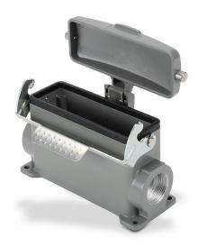
ZIPport surface mount housing, single lever, standard, connector housing size 24B, (2) Pg 21 threaded holes, high construction, heavy-duty die cast aluminum. For use with ZIPport size 24B 2-peg connector housings.
