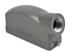
ZIPport hood housing, 2-peg, side entry, connector housing size 24B, (1) Pg 21 threaded hole, heavy-duty die cast aluminum. For use with ZIPport size 24B single lever connector housings.
