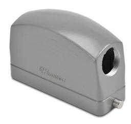
ZIPport hood housing, 2-peg, side entry, connector housing size 24B, (1) Pg 21 threaded hole, high construction, heavy-duty die cast aluminum. For use with ZIPport size 24B single lever connector housings.
