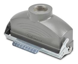
ZIPport coupler housing, single lever, connector housing size 24B, (1) Pg 21 threaded hole, heavy-duty die cast aluminum. For use with ZIPport size 24B 2-peg connector housings.
