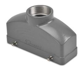
ZIPport hood housing, 4-peg, top entry, connector housing size 24B, (1) Pg 29 threaded hole, heavy-duty die cast aluminum. For use with ZIPport size 24B double lever connector housings.
