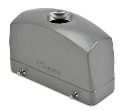
ZIPport hood housing, 4-peg, top entry, connector housing size 24B, (1) Pg 21 threaded hole, high construction, heavy-duty die cast aluminum. For use with ZIPport size 24B double lever connector housings.
