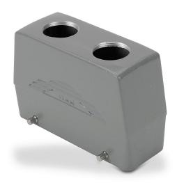
ZIPport hood housing, 4-peg, top entry, connector housing size 24B, (2) Pg 21 threaded hole, high construction, heavy-duty die cast aluminum. For use with ZIPport size 24B double lever connector housings.
