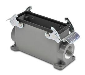
ZIPport surface mount housing, double lever, connector housing size 24B, (2) Pg 21 threaded holes, high construction, heavy-duty die cast aluminum. For use with ZIPport size 24B 4-peg connector housings.
