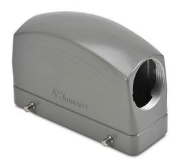
ZIPport hood housing, 4-peg, side entry, connector housing size 24B, (1) Pg 29 threaded hole, high construction, heavy-duty die cast aluminum. For use with ZIPport size 24B double lever connector housings.
