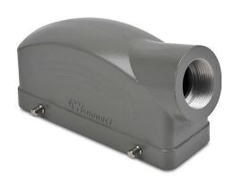
ZIPport hood housing, 4-peg, side entry, connector housing size 24B, (1) Pg 21 threaded hole, heavy-duty die cast aluminum. For use with ZIPport size 24B double lever connector housings.
