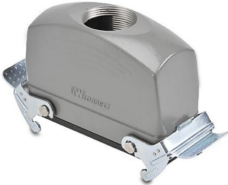
ZIPport coupler housing, double lever, connector housing size 24B, (1) Pg 29 threaded hole, high construction, heavy-duty die cast aluminum. For use with ZIPport size 24B 4-peg connector housings.
