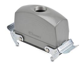
ZIPport coupler housing, double lever, connector housing size 24B, (1) Pg 21 threaded hole, high construction, heavy-duty die cast aluminum. For use with ZIPport size 24B 4-peg connector housings.
