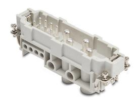
ZIPport male insert, connector housing size 24B, 12-pole, screw terminals, accepts wire size 6 - 16 AWG, 20 - 14 AWG, 80 amp (4-pole), 16 amp (8-pole), 600 VAC/VDC, poles numbered 1 to 4 and 1 to 8. For use with ZIPport multi-wire housings.
